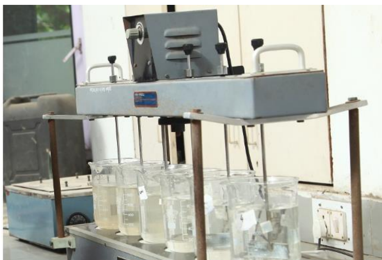
Project on Jar testing equipment for chemical treatment
