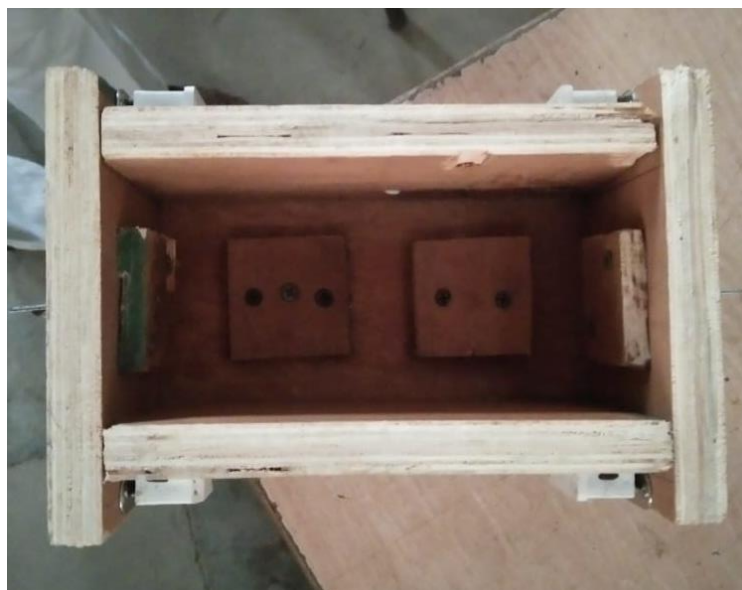
Project on making grooved brick mould and samples
